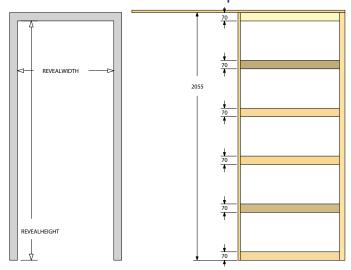
Pressed metal sliding door frame installed with a timber pocket for heavy duty cavity unit that are easy to assemble.
